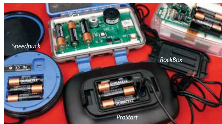
The Velocitek SpeedPuck and ProStart have sealed innards, but the Velocitek SC-1 and RockBox bare their circuit-board souls.
