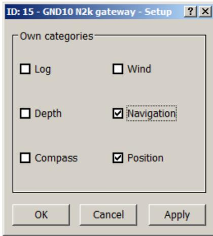
In the example above, a NX2 Server is used and the Log, Depth, Wind and Compass will all come from the Nexus transducers. GPS Position and Navigation data will come from the NMEA2000 network and be send out on the Nexus Network. Log, Depth, Wind and Compass will be send out on the NMEA2000 network from the GND10.
