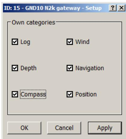
As you can see all tick boxes are checked and the GND10 will convert NMEA2000 data and send it out on the Nexus Network. For the transducers/functions you want the Nexus Network to provide for, un-check the equivalent box:
